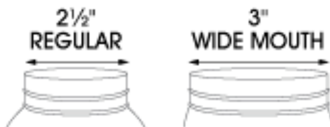
Figure 2. Uline Canada’s Different Sizes of Mouths Offered on All Sizes of Glass Canning Jars Sold (Regular Mouth- 2.5 “ and Wide Mouth- 3 “) (ULINE, n.d.)
